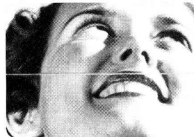
When the halves of the image have been brought into register, as they appear here, the lens is in exact focus for the subject.
