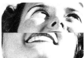
Here the halves are out of alignment because the lens is focused for a distance greater than that from the camera to the subject.
